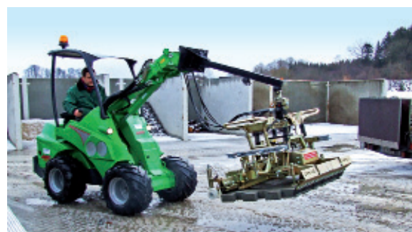
Installation clamp in combination with Mini-excavator
