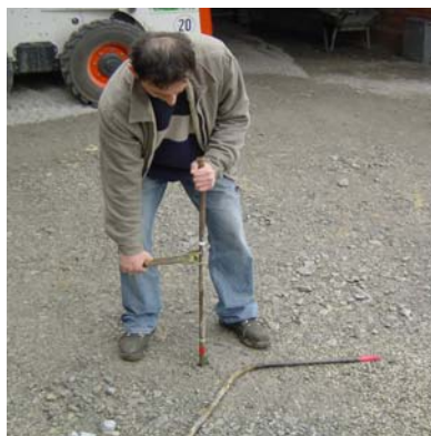
When lifted up, the V-shaped clamping system locks to the pin. Now pulling and turning movements to loosen the pin, can be executed without any real physical effort
