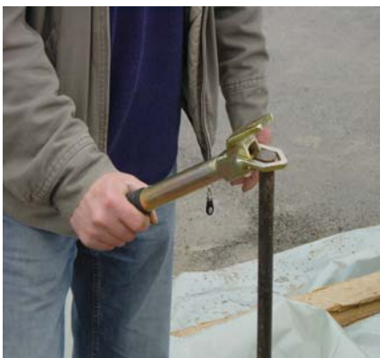
Pin Extractor ENZ is simply put over the top end of the pin
