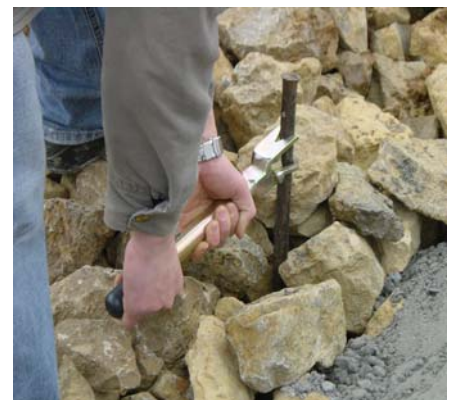
The tool also works when the pin is only sticking out a few centimetres of the ground
